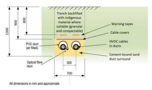
Figure 6 Typical HVDC Trench Cross-Section (source: WSP | not to scale)
