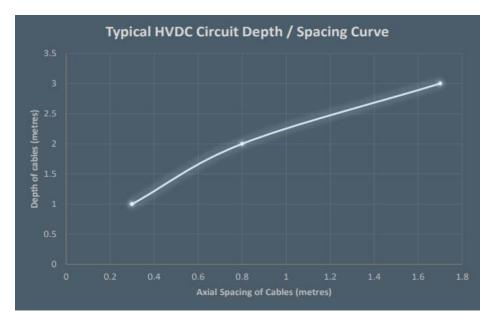
Figure 7: Typical HVDC Circuit Depth/Spacing Curve
