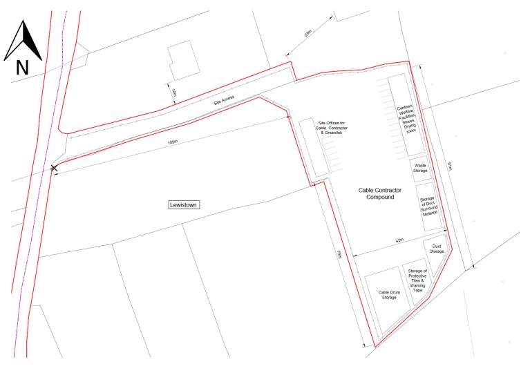
Figure 4.4 Contractor's Compound at Lewistown | not to scale
