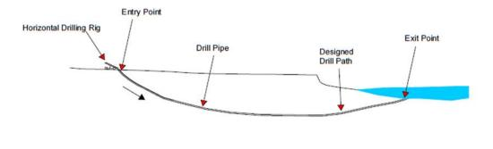
A small diameter pilot hole is drilled from the entry point, under the sea bed, to the exit point.
