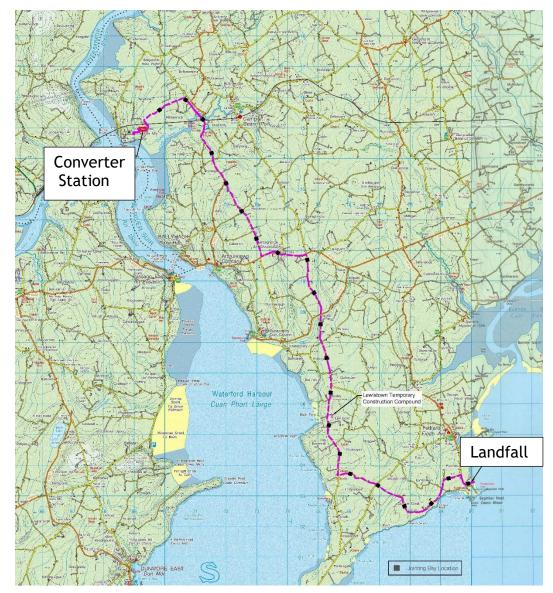
Figure 4.11: provisional Jointing Bay Locations | not to scale
