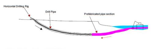
Prefabricated pipe is attached to a swivel behind the Reamer and pulled into place under the beach
